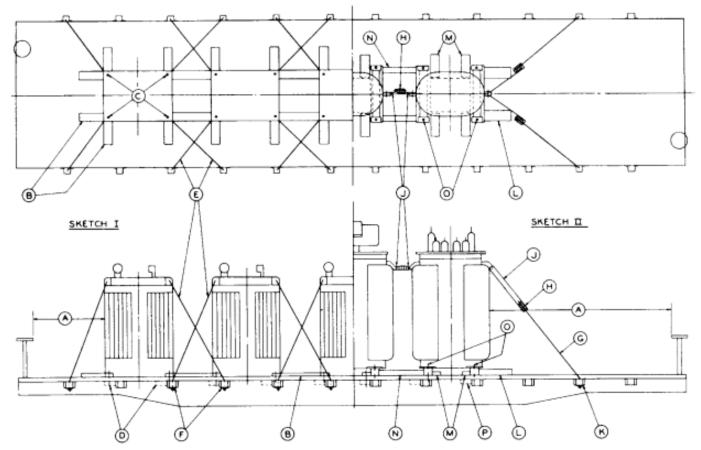
TRANSFORMERS, TRANSFORMER TANKS, CIRCUIT BREAKERS AND SIMILAR UNITS, 35,000 LB OR LESS-FLATCARS
